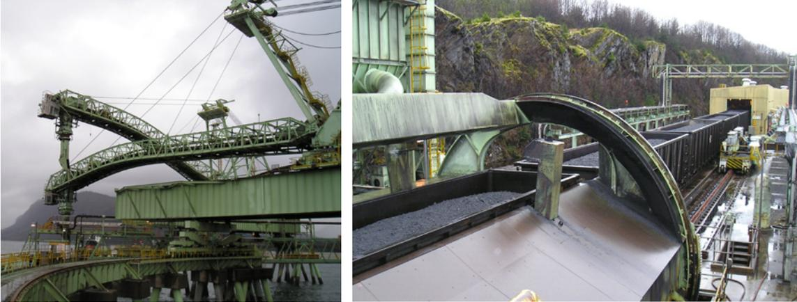
*Continuous rotary rail car dumper and coal transfer at Prince Rupert*
